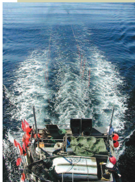
Longline gear being set with streamers to prevent seabirds from being caught
